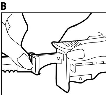
**IMPORTANT:** Unplug and be sure the Safety Button is in the "Lock" position before inserting or removing Blades. In this position, the Operating Bar cannot be pressed in even when the Knife is plugged in. (A).
