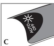
4. Plug in the iron. The on indicator light illuminates green (C). Once the iron reaches the selected temperature, the light goes off and stays off during the ironing cycle.
