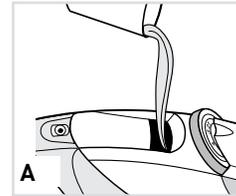
1. Tilt the iron and using a clean measuring cup, pour water into water-fill opening (A) until the water reaches the MAX mark on the water tank. Refill as needed.
