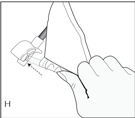
5. Insert the transparent tube into the latch of the curved tube end on both ends of the kabana (H).
